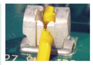
soldering wires to the PCB. It was also designed to be automated by the customer's existing pick and place equipment using standard taping methods. This is a surface mount version of a proven through-hole connector. It is re-usable, has a low profile, and is geographically stable. Our family of SMT IDCs can terminate a large range of stranded or solid wire gauges.
