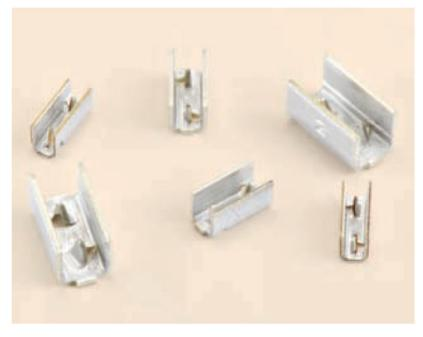
contact spikes protrude from the flat base. Between the contact spikes there is a flat area to facilitate vacuum pick-up and terminal placement. There are two deep score lines near the transition area between the side wall and the base of the terminal.
